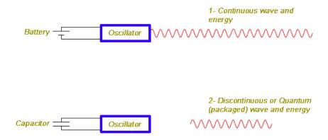
In figure 1, the battery supplies energy of oscillator runs continuously. Consequently, the oscillator will produce radio waves until finishing battery charge.
